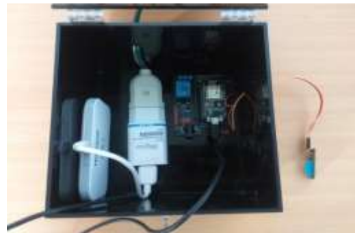
Gambar 5. Alat Monitoring Bearing Scavenge Temperature Berbasis Internet Of Things (IOT).
