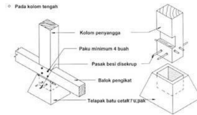
Gambar 6 Pondasi Umpak
